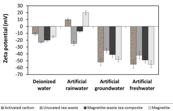
**Figure 7.  $\zeta$ -potentials of the various sorbents dispersed in the artificial waters.**
