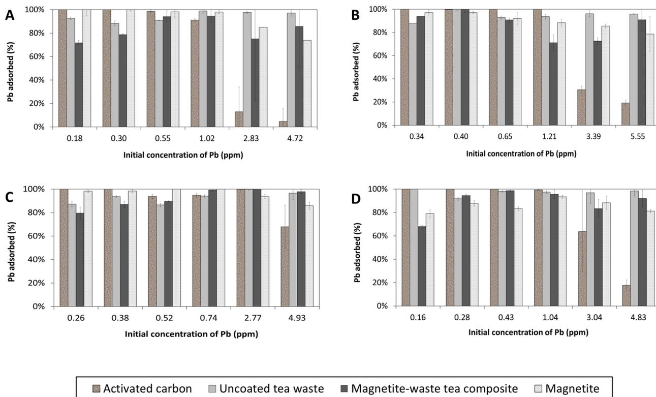
**Figure 6. Percentage of Pb adsorbed onto the four sorbents for each of the four different waters: (A) deionized water, (B) rainwater, (C) groundwater and (D) freshwater.**
