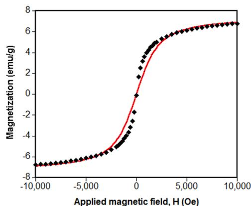
**Figure 3.** Magnetization curve of the magnetite-waste tea composite at room temperature. The points were obtained from VSM measurement, while the solid line was the best fit from the Langevin function assuming the composite particles were monodisperse.
