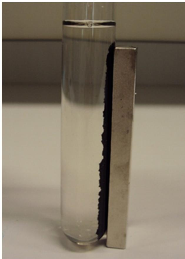
**Figure 4. Testing the magnetic stability of magnetite-waste tea composite after 8 days in water.**
