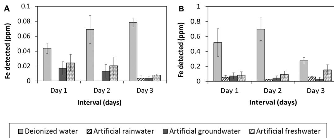
**Figure 5. Amount of Fe leached out into the four waters from uncoated tea (A) and magnetite-waste tea composite (B).**
