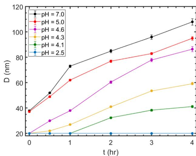
**Fig. 8.** The stability of the nanoemulsion at room temperature as a function of pH by monitoring the nanoemulsion droplet size over time. pH was adjusted using NaOH. See Fig. S4 for a long-time droplet size monitoring. The error bars are standard errors from 15 measurements.
