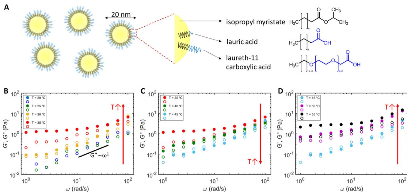
**Fig. 1.** Schematic of the nanoemulsion suspension and the linear viscoelastic moduli (closed:  $G'$ , open:  $G''$ ) as a function of angular frequency ( $\omega$ ) at elevated temperatures. The pH of the nanoemulsion is 2.5. (A) The schematic of the nanoemulsion suspension. Upon increasing the temperature, viscoelastic moduli (B) first increase, (C) then decrease, and (D) finally increase again.
