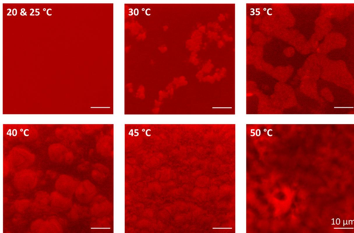
**Fig. 3.** Microstructures of the nanoemulsion (pH = 2.5) at elevated temperatures using confocal microscopy. The oil droplets are fluorescently labeled using Nile Red. Scale bars = 10  $\mu\text{m}$ . (For interpretation of the references to colour in this figure legend, the reader is referred to the web version of this article.)
