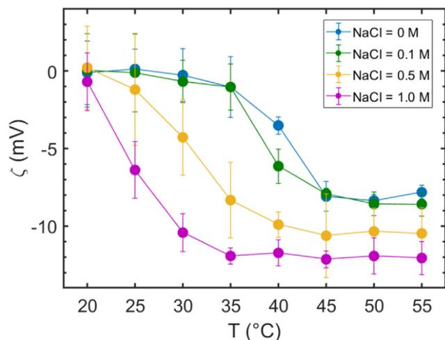
**Fig. 10.** Zeta potential ( $\zeta$ ) of the nanoemulsion droplets as a function of temperature ( $T$ ) at elevated ionic strength. Ionic strength was adjusted using NaCl. The pH of the nanoemulsion is 3.1. The error bars are standard errors from 30 measurements.
