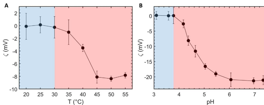
**Fig. 5.** Zeta potential ( $\zeta$ ) of the nanoemulsion droplets as a function of (A) temperature,  $T$  and (B) pH at  $T = 20^\circ\text{C}$ . pH was adjusted using NaOH. The pH of the nanoemulsion in (A) is 3.1. The error bars are standard errors from 30 measurements.
