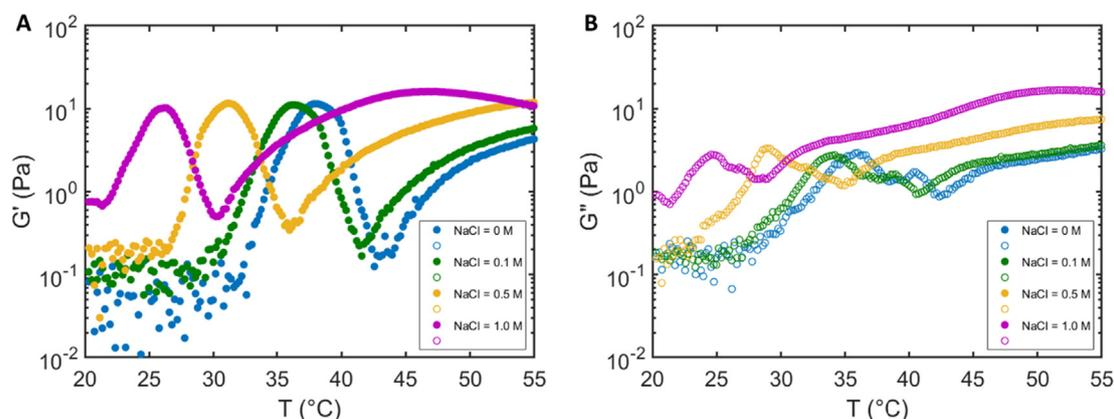
**Fig. 9.** Effect of the ionic strength on the rheological properties of the nanoemulsion (pH = 2.5) using SAOS at a fixed angular frequency = 25 rad/s. The figure shows (A) storage modulus,  $G'$  and (B) loss modulus,  $G''$  as a function of temperature,  $T$ , with increasing ionic strengths. The ionic strength was adjusted using NaCl as indicated in the figure.
