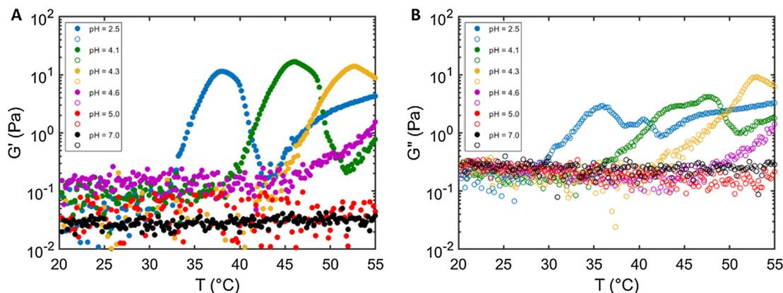
**Fig. 7.** Effect of pH on the rheological properties of the nanoemulsion using SAOS at a fixed angular frequency = 25 rad/s. The figure shows (A) storage modulus,  $G'$  and (B) loss modulus,  $G''$  as a function of temperature,  $T$ , at various pH values. pH was adjusted using NaOH.
