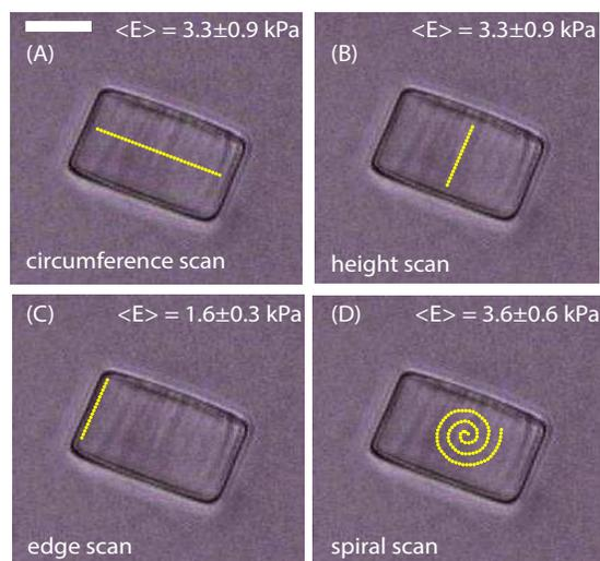
**Fig. 2** Hydrogel cylinders of diameter 48  $\mu\text{m}$  and height 30  $\mu\text{m}$  were probed along the (A) circumference (B) height (C) edge and (D) in a spiral manner. The scale bar is 20  $\mu\text{m}$ .
