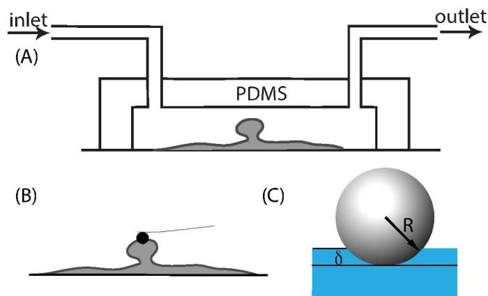
**Fig. 1** (A) Experimental set up of the flow cell showing the biofilm growing on the glass surface of the chamber. (B) AFM cantilever with a spherical polystyrene tip of radius 5  $\mu\text{m}$  was used to probe the surface of the biofilm. (C) The Young's modulus was measured from the indentation depth for a given force.
